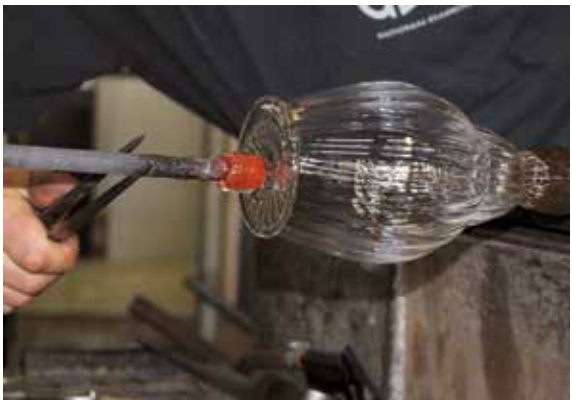
13) The pontil or pointy, a solid metal rod with a small bit of glass on the end, is attached to the base of the piece.
