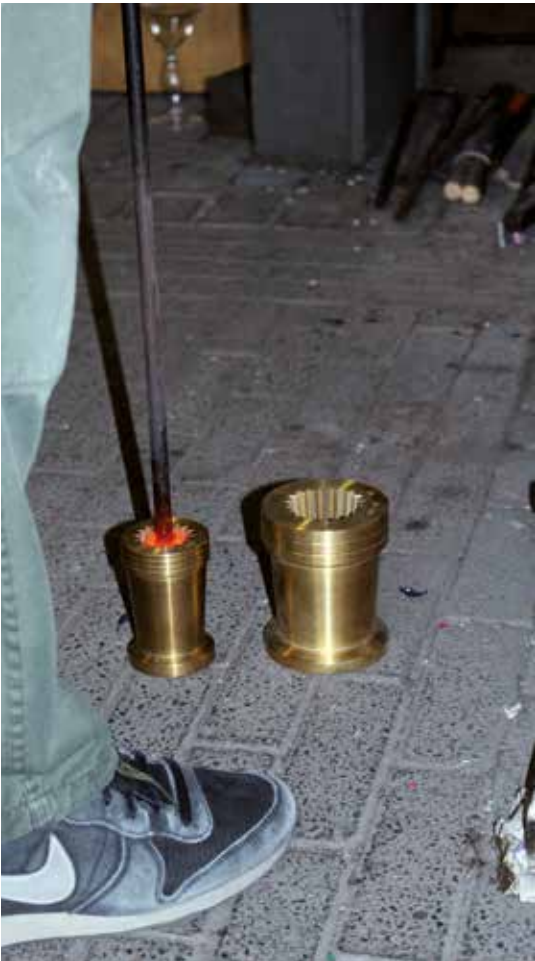
1) After picking up some blue glass from the oven, the glassblowers rolls it on the marver and blows some air in it until it fits exactly into the mould. Then he puts it in the small mould and blows as hard as he can to force the glass into the form of the mould.
