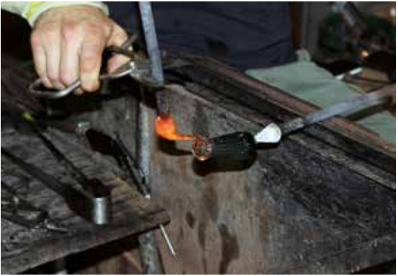
17) After the first assistant picks up the ball from the annealing oven, and while the second assistant reheats the vase to maintain temperature, the ball is brought to the master. The first assistant brings a bit of glass and the glassblower adds a glass thread around the base of the ball to be able to attach the ball to the inside of the vase.
