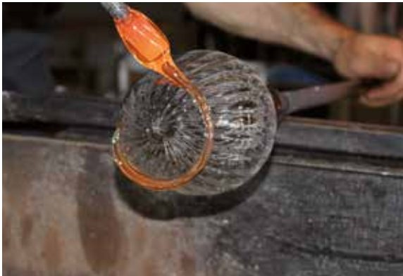
11) The assistant brings a bit of glass on the end of a punty iron. The glassblower puts it onto the glass holding the iron with his tweezers. By turning the glass he draws a glass thread onto the rim of the base, making a footrim.
