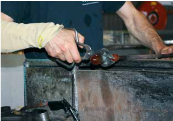
2,3) The glassblower shapes the ball whilst the first assistant blows.
