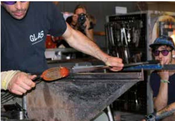
7,8) While the first assistant blows, the master shapes the glass
