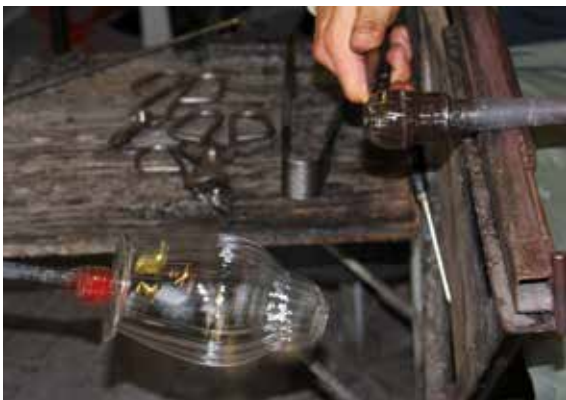
14) The glass is transferred to the punty so that the top of the vessel can be finished.
