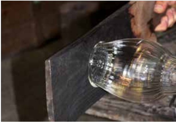
12) The footrim is flattened with a piece of wood
