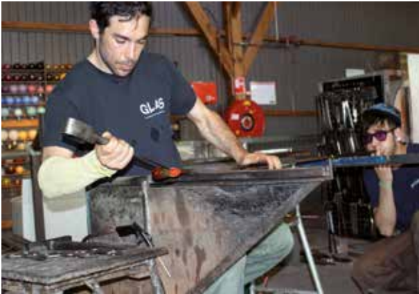
2,3) The glassblower shapes the ball whilst the first assistant blows.
