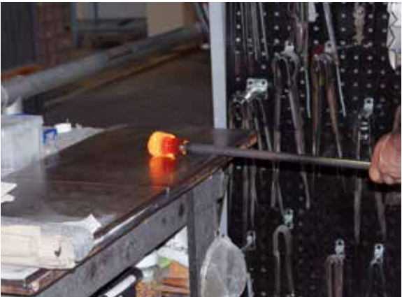
5) After picking up some colourless glass from the oven, the glassblower rolls it on the marver.
