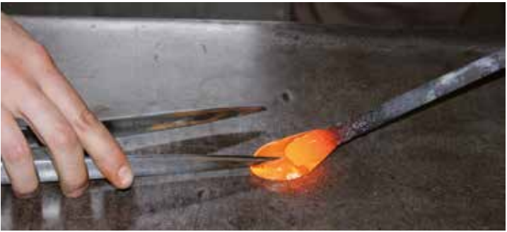
19) To make the handles, first a line is pressed with the tweezers into a bit of glass
