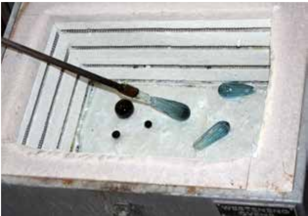
4) The glassblower puts the ball into the garage (holding oven)
