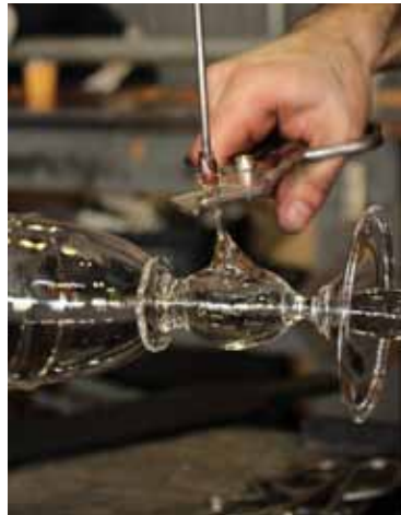
The hot glass is stuck to the rod and pulled with it, shaping the first spout. These steps are repeated twice, to make two other spouts.
