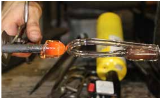
The assistant brings a punty with a small gather of glass and sticks it onto the siphon. The master cuts it loose.
