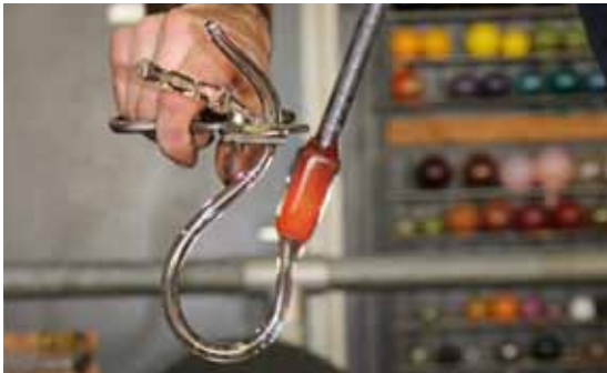
To make the siphon, the glassblower blows a thin, long bubble. He bends it into the shape of the siphon.
