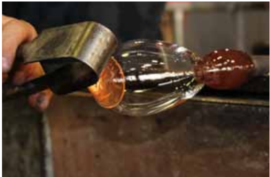
The glassblower blows a bubble to make the bowl of the glass. An assistant brings a gather of glass on the end of a steel rod called an "iron" or "gathering iron". The master covers the base of the glass with it.
