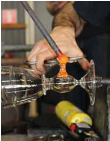
In order to make a spout on the stem, the assistant brings a gather of glass that is added to the side of the hollow stem.
