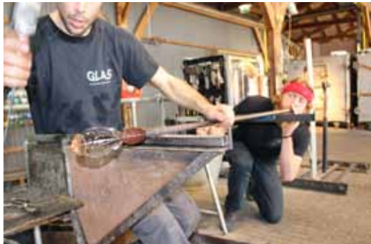
The assistant blows into the blowpipe, forcing air through the base of the bowl into the hot bit of glass, forming a second bubble.
