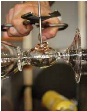
The master pushes a thin steel rod into and through the hot glass on the stem. He now pulls the rod out.
