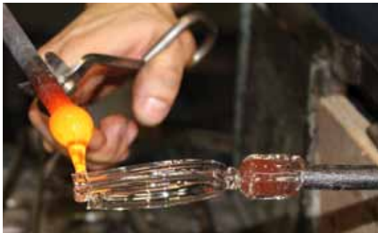
The master adds a glass thread around the end of the siphon that will be fused around the hole in the base of the bowl.
