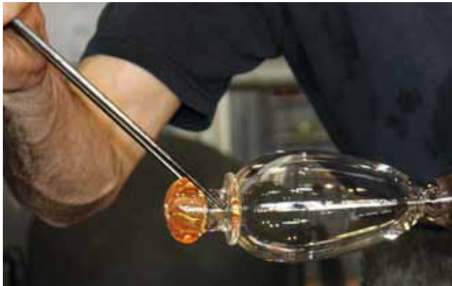
While the assistant blows, the master shapes this bubble into the stem of the glass.
