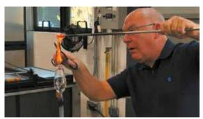
6) Preformed canes of colored glass are attached to the surface to a gather of molten glass. This is then attached to the tip of the ball-shaped tip at the base of the cup. Using shears, the nascent stem is cut free of its gathering rod.
