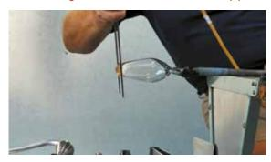
4) As the two-bladed tool called 'the jacks' is used to squeeze a portion of the soft glass to create a disc-like merese, air is blown forcefully into the blowpipe. The still-soft glass at the tip, having re-softened the vessel-wall inflates slightly.
