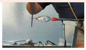
2) As the glass is further inflated, the tip is pulled to elongate the bubble and to make the lowermost part of the cup conical in shape. A constriction is formed near the blowpipe. Later in the process (see fig. 15 below) this will allow the goblet to be broken free of the blowpipe.
