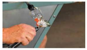
12) Small gathers of transparent aquamarine glass are added to the sides of the stem, then manipulated using pincers having a waffle-pattern on their working-surfaces.
