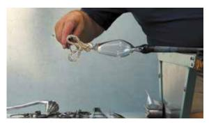
10) The outermost area of the loop is pushed inward toward the blowpipe.
