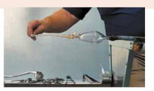
8) The pincers (tweezers) are used to pull the loop outward as the blowpipe is turned. This forms a long, spiraling 'cable'.
