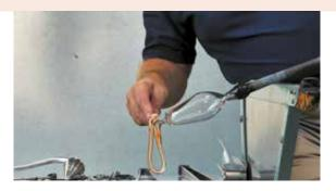
7) The tip of the stem is pulled outward, then its end is quickly stuck near its first contact-point, thus forming a loop.
