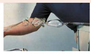
14) A hole is made in the end of the bubble, and after reheating the glass the jacks are used to create a folded edge and then give the foot its final shape.
