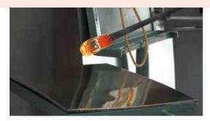
1) The process begins with a gather of molten glass on the end of a metal blowpipe. This partially inflated bubble will become the cup of the goblet.
