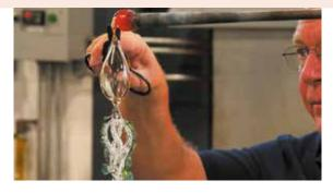
13) After the lowermost part of the stem is created, a soft bubble of glass is lowered onto and attached to its tip. This will become the foot of the goblet.
