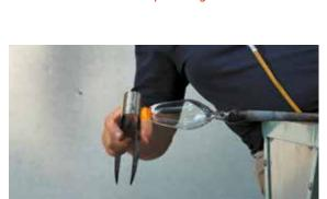
3) A small gather of molten glass is added to the tip of the cup and flattened.
