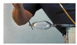
5) The small bulge of inflated glass is given a constriction and pulled outward using the jacks. As the ball thus formed is pulled outward, the cavity of the vessel is also elongated, leaving the tapering constriction hollow.
