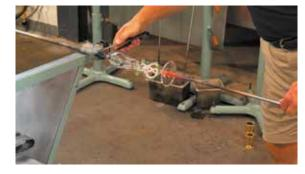
15) The goblet is transferred to a pontil (or 'punty'), a metal rod with a small amount of molten glass on its hot end; this acts as a handle for the conclusion of the manufacturing process. The constriction near the blowpipe (see fig. 2 above) is broken.
