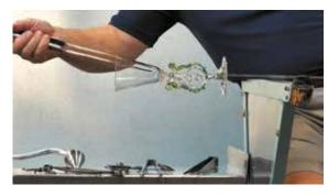
16) After reheating the uppermost part of the cup, the jacks and soffietta (a conical metal inflating-tool) are used to give the cup its final form.
